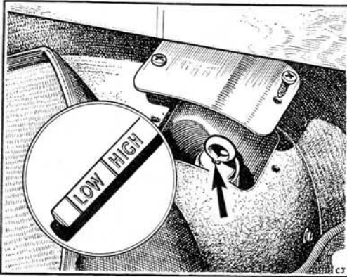
Fig. P.11. The gearbox dipstick.
